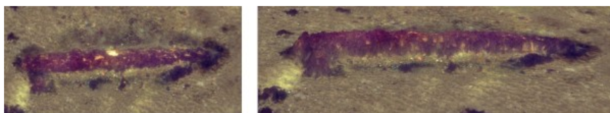
Figure 4: 3D reconstruction from several hundred photos of a torpedo (GEOMAR). Left: top view. Right: side view.
